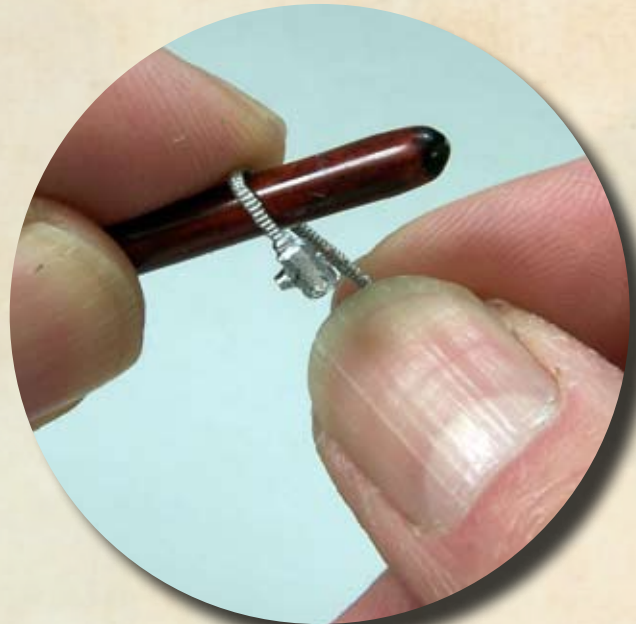
Above & below. To save stress on the cable I slowly bent it around an old paintbrush.
